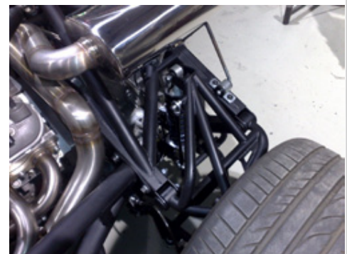
Rear Suspension Designed with ADAMS
