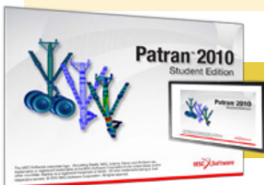
Figure 7 Patran Student Version Limited to 5000 nodes, 1000 curves & 500 surfaces and 100 solids
