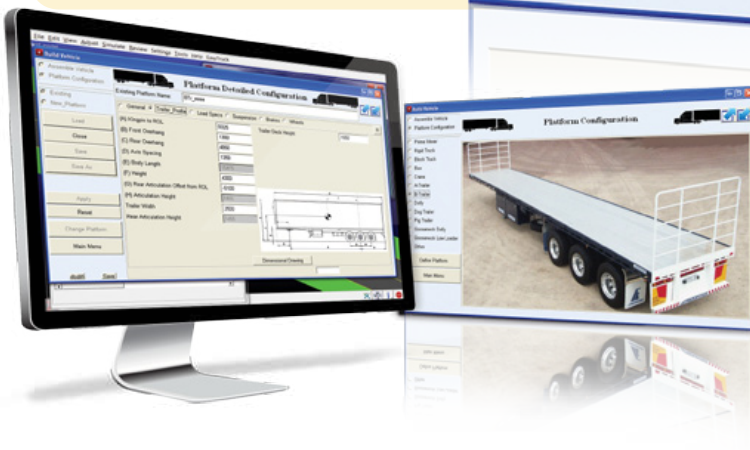
Figure 4 Example of platform configuration for a B-Trailer
